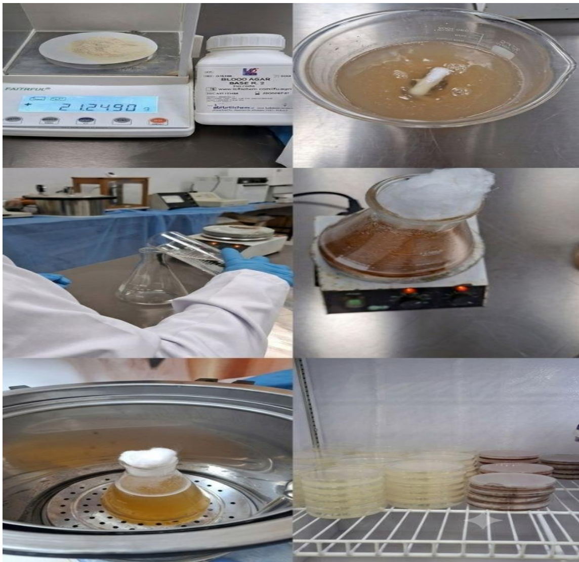
Figure 3: Laboratory preparation of culture media, sterilization, and agar plate pouring for bacterial isolation.
